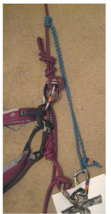
← Step 2: Attach a prusik hitch to the rope and clip it into the anchor. Use only a perlon (nylon). Spectra melts at too low a temperature for friction hitches.
