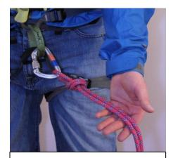
1) Attach to the rope at the predetermined distance from center person with a figure 8 on a bite and a locking carabiner
