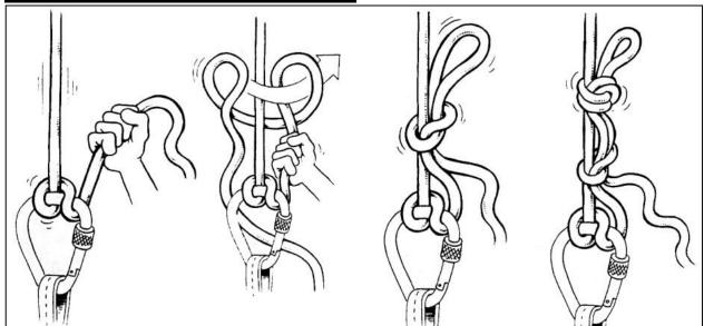
This combination can be used to tie off a loaded rope. It can also be used in place of a Mariner knot when using a cordelette.
