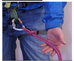
1. Attach to the rope at the predetermined distance from center person with a figure-8 on a bite and a locking carabiner.
