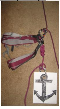
← **Step 0:** Fall is arrested (belayer omitted for clarity).
